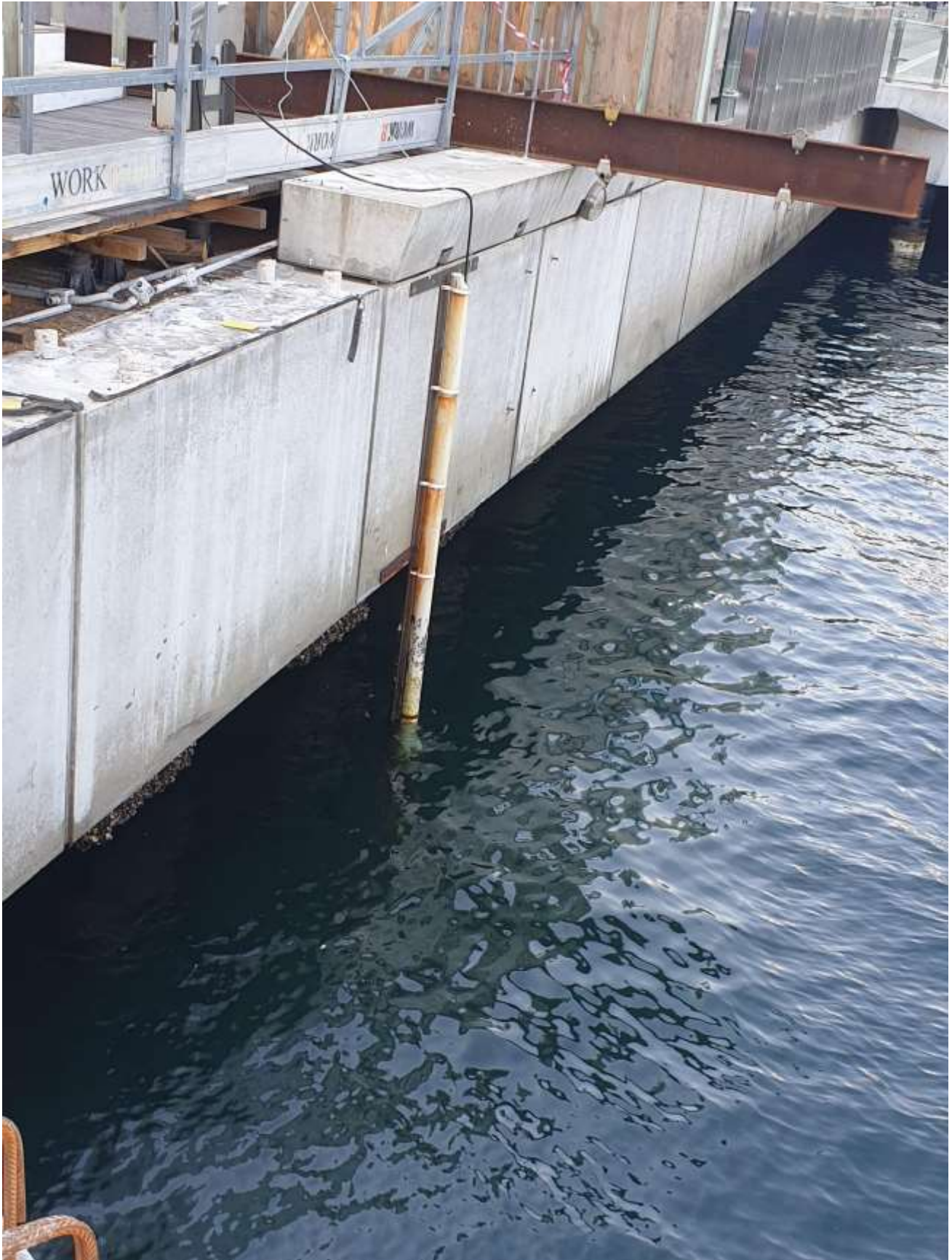
Photo 12: Water quality monitoring probe
